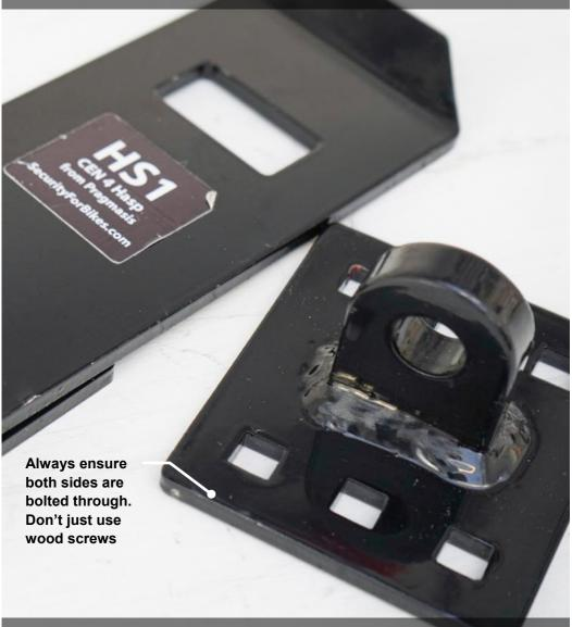
Quality hasp sets have a vertical staple eye. This allows a closed shackle padlock to hang properly. A horizontal eye means a closed shackle lock will protrude outwards making it more vulnerable to attack with a hammer.
